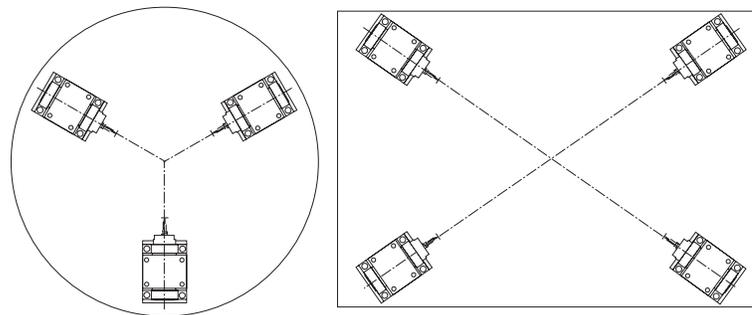
Recommended weigh module orientation in order to give self locking conditions and freedom for mechanical movements caused by temperature.
